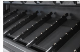
Pneumatic Backgauge Support (ball bearing slide plate)
