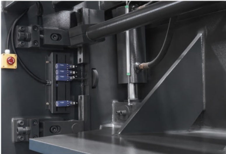
Adjust Blade Clearance With Upper Fulcrum
