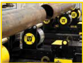
Pipe loaded, lined up using track drive.
