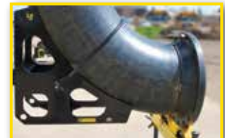
Fasten elbow into the jig.
