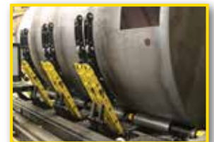
Side Jigs to eliminate thin-wall vessel sagging.
