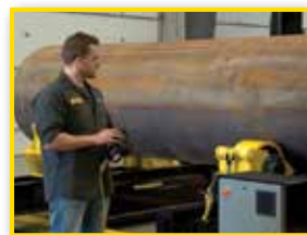
Alignment, leveling and high/lows easily adjustable using pendant or touch screen control.
