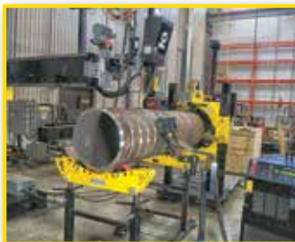
Optional fully integrated rolling induction heating systems.
