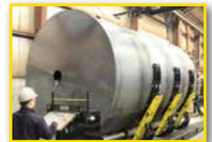
Integration with automated LJ welding manipulators.
