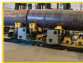
Sections brought together using powered track drive.
