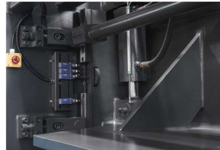
Adjust Blade Clearance With Upper Fulcrum
