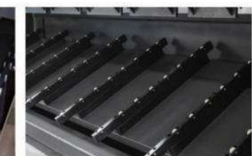
Pneumatic Backgauge Support (ball bearing slide plate)
