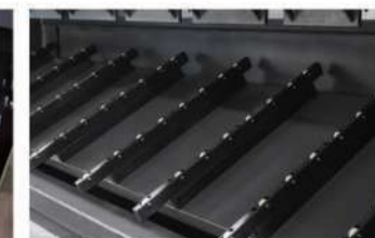
Pneumatic Backgauge Support (ball bearing slide plate)
