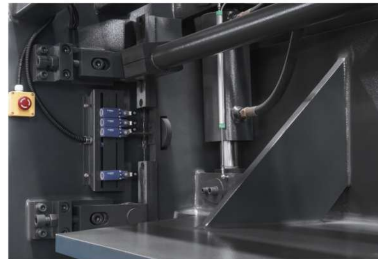
Adjust Blade Clearance With Upper Fulcrum
