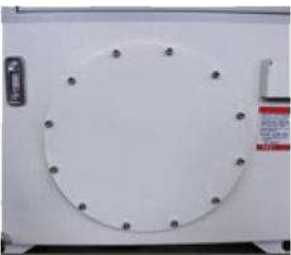
Hydraulic Oil Tank
