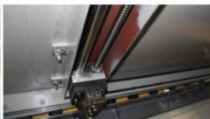
X-axis Ball Screw And Grinding Light Rod
