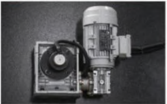
Electric Adjustment of Blade Clearance
