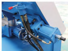
● Saw blade hydraulic clamping
