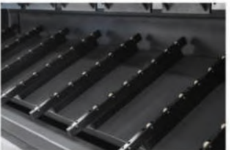
Pneumatic Backgauge Support (ball bearing slide plate)
