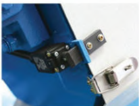
● Protective cover power failure protection
