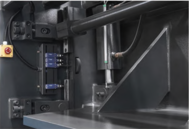
Adjust Blade Clearance With Upper Fulcrum
